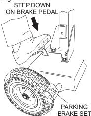
Figure 8. Parking Brake (Set Position)
